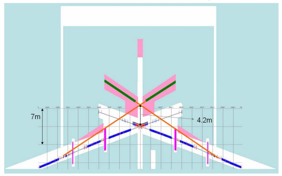
additional angle is 5.5mrad and detector need to move by about 4.2m
