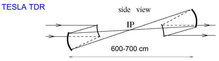
Then the diameter of focusing mirror is about 20 cm and that of the auxiliary mirror about 11 cm. The dead angle for tracking remains as before about ±95 mrad, for calorimetry smaller. The laser density is far from the damage threshold, the average power is the most serious problem.
