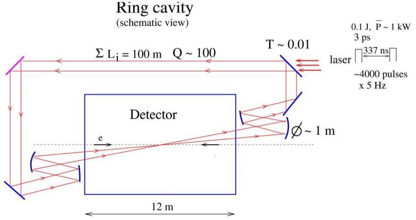
The cavity includes adaptive mirrors and diagnostics. Optimum angular divergence of the laser beam is  $\pm 30$  mrad, A≈9 J (k=1),  $\sigma_t \approx 1.3$  ps,  $\sigma_{x,L} \sim 7$  µm
