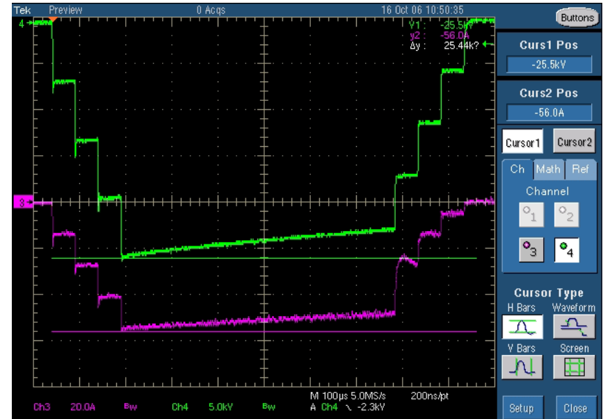
4-Cell Output Waveforms : ~25kV, 600µs
