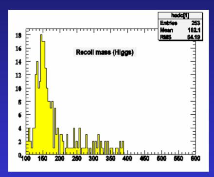
Geometry acceptance (Efficiency) of the LDC detector is very high 98% (3events from 256) for the muons channel of Z decay
