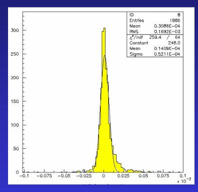
Momentum reconstruction resolution for barel and endcup tracking for muons 30 GeV: central region 4.7x10<sup>-5</sup>, forward region 5.2x10<sup>-5</sup>
