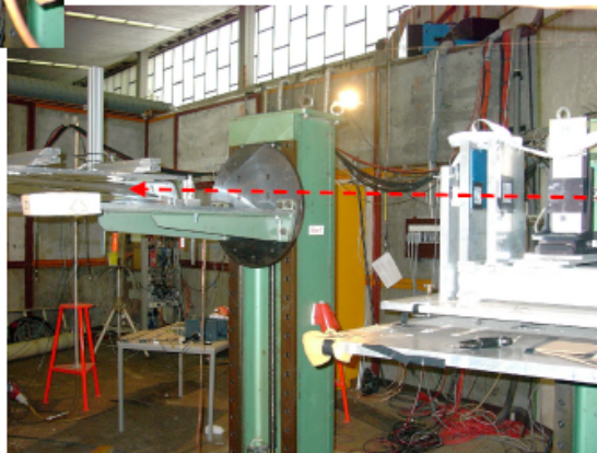
Test set-up 2: One GLAST module Read out by VA1&180nmUMC
