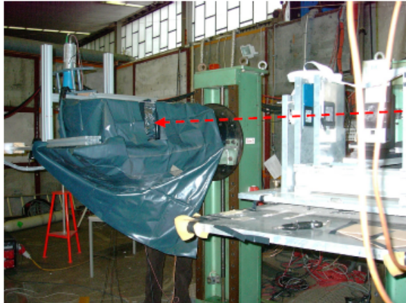
Test set-up 1: Two CMS modules First one read out by 4VA1 Second one read out by VA1&180nmUMC
