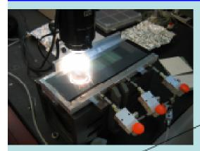
Assembly 3 CMS sensors 28 cm strip long Read out: VA1+180UMC r.o and all VA1 r.o.
