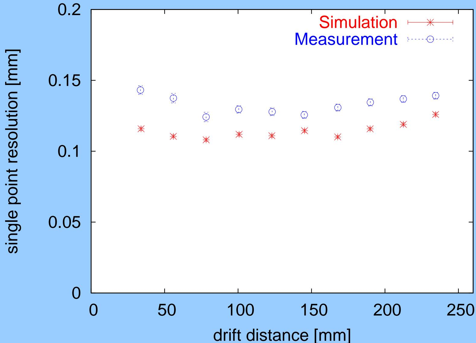
8 bit ADC, 12.5 MHz, P5 Gas, 0T, DESY Testbeam
