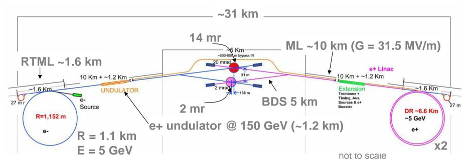
Configuration used for Vancouver cost estimate fundamentally no different from Frascati BC, but much more detail design work
