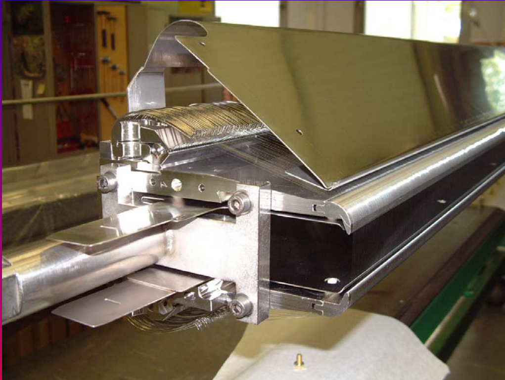
SPS ZS anode with the ion traps on the assembly bench
