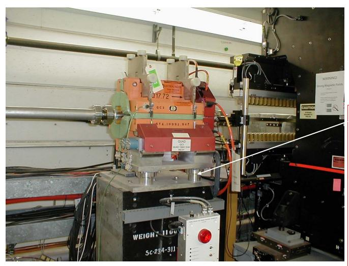
This support has to be redesigned to be much shorter, so magnet center will be at desired height in ATF2.
