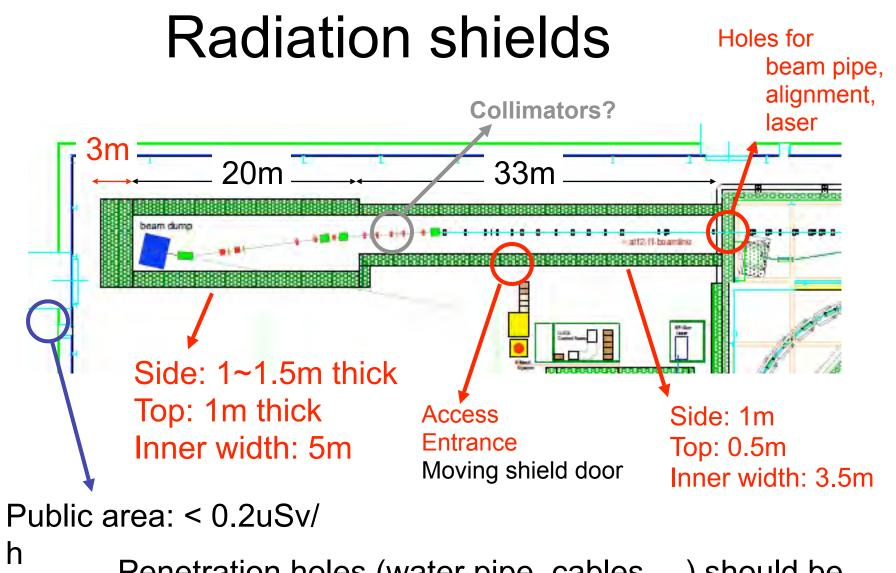
Penetration holes (water pipe, cables,...) should be well designed.
