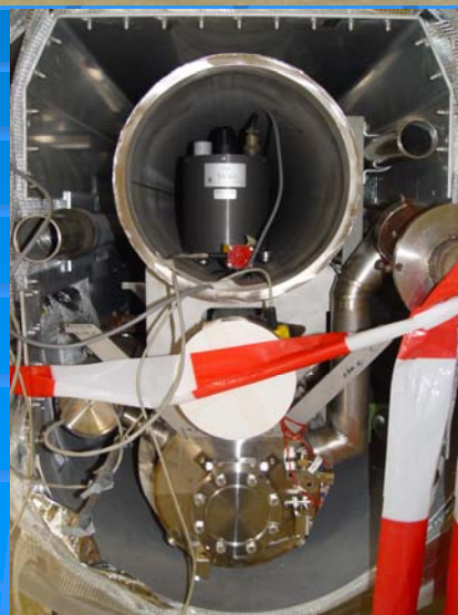
Seismometer Guralp CMG-6TD inside Helium Gas Return Pipe (GRP)
