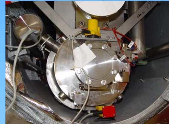
Sensor SM-6 vertical geophone placed on the cryostat
