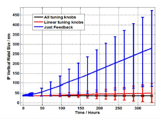
At each point, none, linear (waist, dispersion and coupling) and full tuning knobs (include sextupole strength and tilt scans) applied. For blue, red and black respectively.
