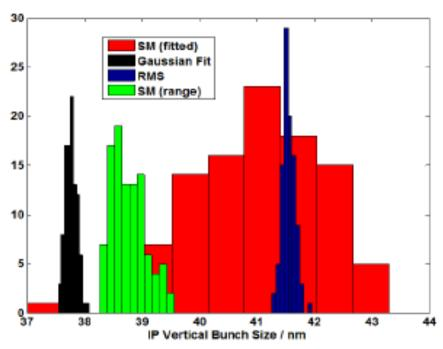
Can measure (in simulation) the beam size in different ways with different results (at 10% level).
