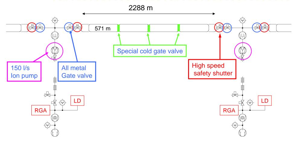
2 TMP pumping units with high sensitivity LD and RGA, safety, clean venting system, slow start pumping etc.
