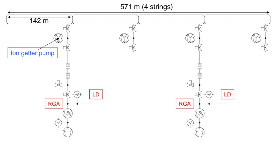
2 TMP pumping units with high sensitivity LD and RGA, safety, clean venting system, slow start pumping etc.
