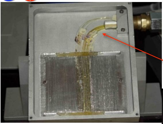
8 100 micron fibers 8 600 micron fibers (one cut at entry) I mm pitch
