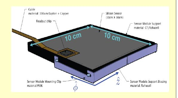
Would require development of 2000 channel chip w/ bump bonding (should be solved by KPiX development)
