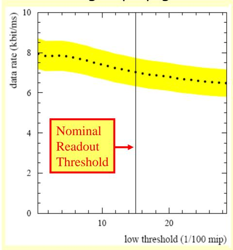
Simulate detector background and noise rates for 500 GeV running, as a function of readout threshold.
