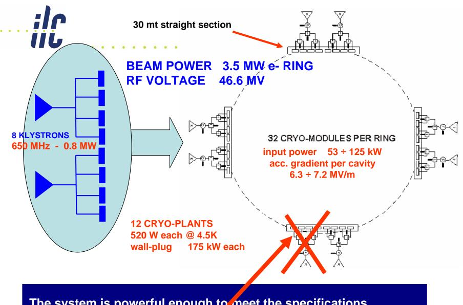
The system is powerful enough to meet the specifications in case of one RF station fault
