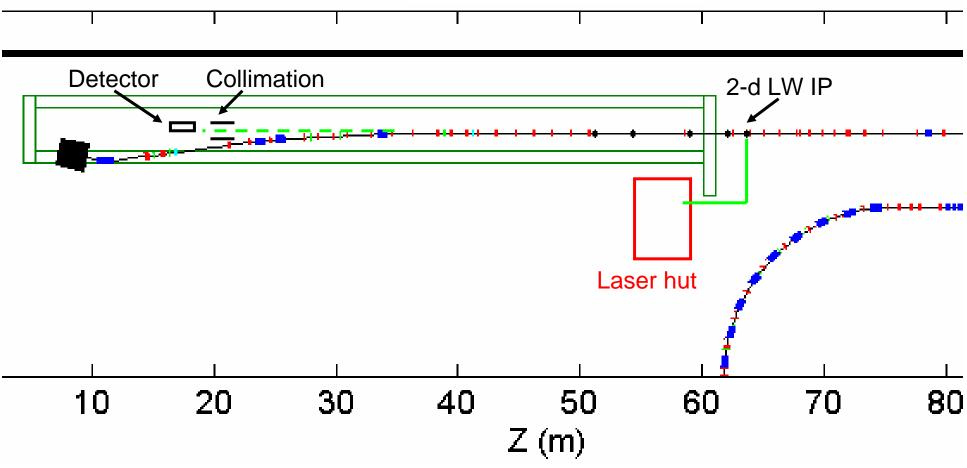
Test design of 2-D IP: if OK, can build additional ones Light path = evacuated 4" pipe, containing relay optics Full Light pipe may need to be installed at stage 1
