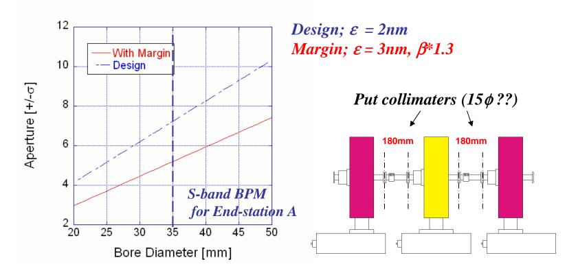
The collimater should be put around SF6 and SF5 for the requirement from the Shintake monitor detector background.
