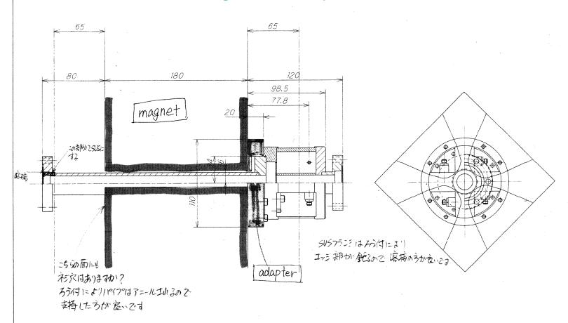
Length of cavity BPM is the magnet length plus 20cm. Furthermore, when we use the 10cm bellows between the cavity BPM, the magnet separation should be the magnet length plus 30cm.
