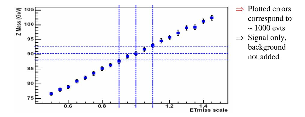
Z mass measured to 3% will result an error of 10% on Missing ET
