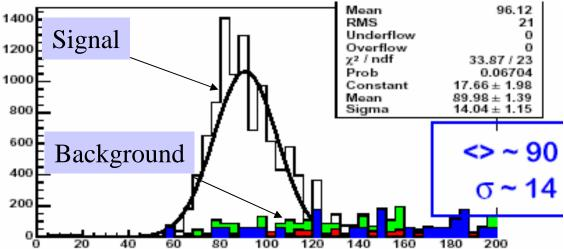
Applied cuts :  $pt(jet) > 25 \ GeV, |\eta| < 2.5$   $pt(lep) > 25/20 \ GeV, |\eta| < 2.5$   $1.<\Delta\phi < 2.7 \ or \ 3.6<\Delta\phi < 5.3$   $m_T(lept-pTmiss) < 50 \ GeV$   $\tau$ -likelihood > 8 ( $\tau$ -eff ~ 30%) No lept isolation
