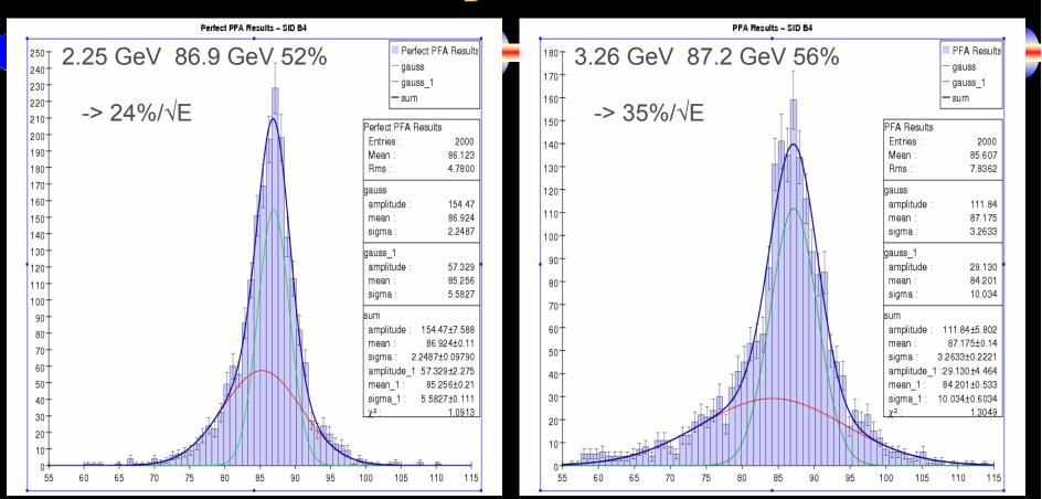
SiD SS/RPC - 5 T field Perfect PFA  $\sigma$  = 2.6 GeV  $PFA \sigma = 3.2 \text{ GeV}$
