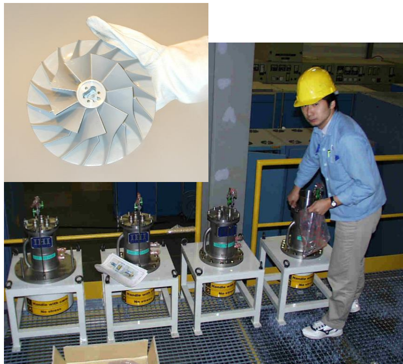
IHI-Linde; 4 cold compressor stages
