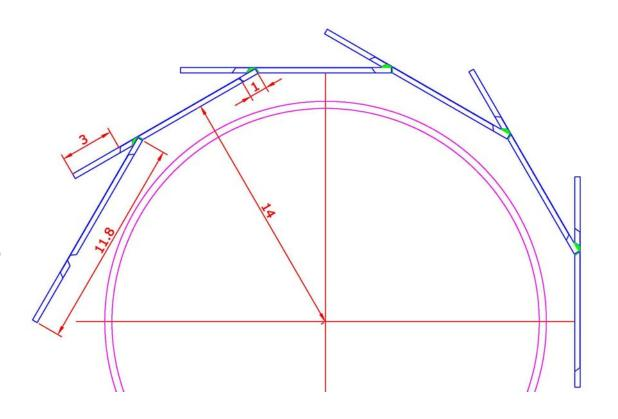
Innermost layer assuming spiral geometry & SiD beam pipe
