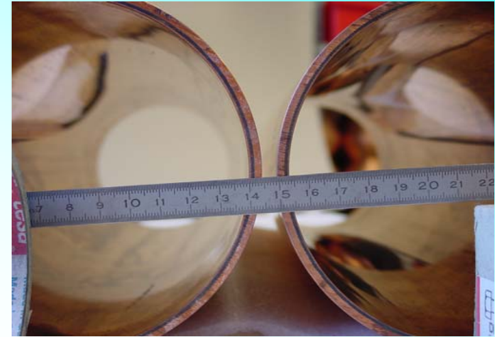
Hot roll bonded Cu-Nb-Cu tube Nippon Steel Co. and KEK
