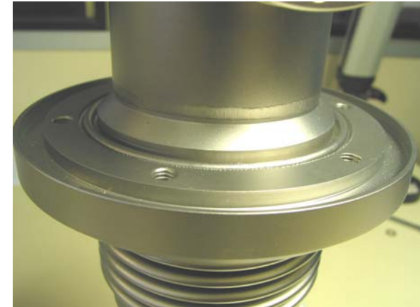
Smooth outer weld
