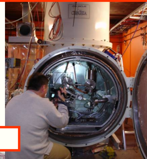
Horizontal Test of Dressed Cavity @ DESY
