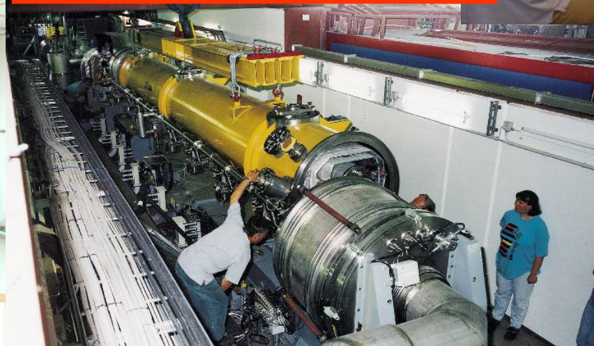
Cryomodule Test at DESY TTF
