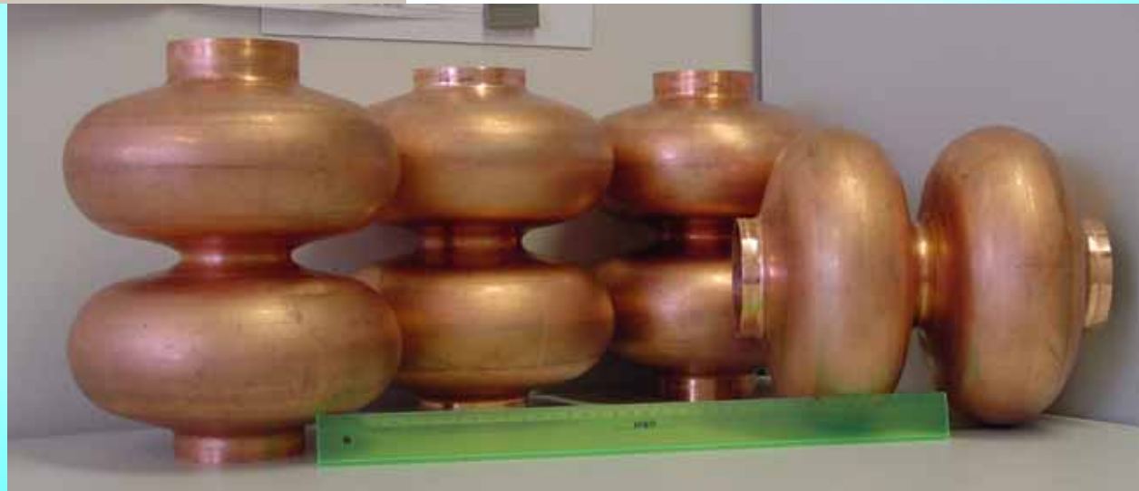
Four 2 cell NbCu clad cavities recently produced at DESY from KEK tubes (no cracks on the inside surface)
