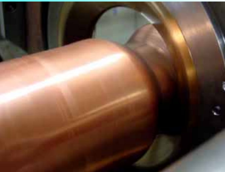
Principle of tube diameter reduction in the iris area
