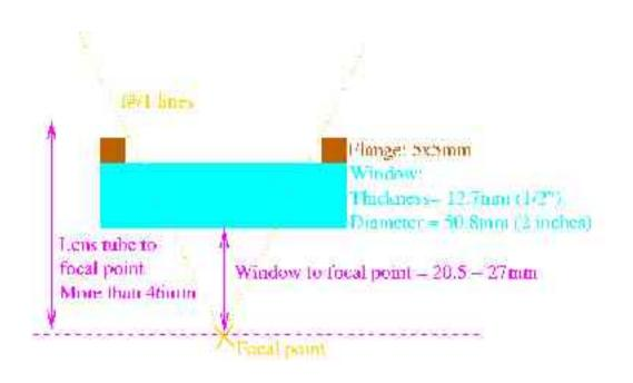
Mechanical constraints on the lens
