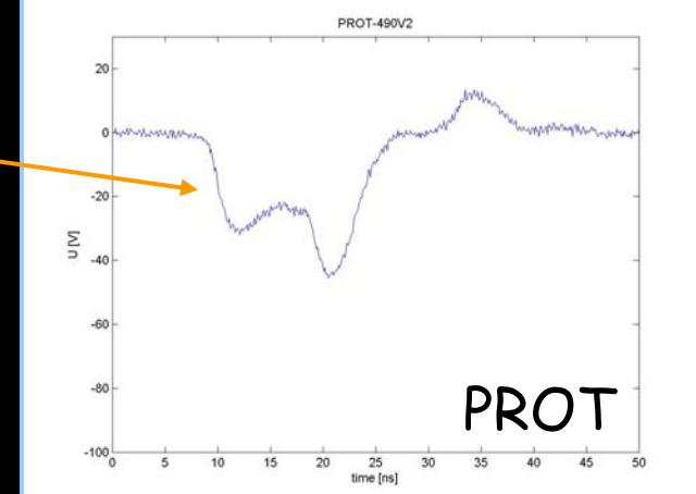
**Slope less steep for protected anode**
