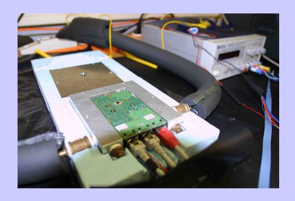
DESY setup enables measurements of the pedestal and the noise distributions and their dependences on a temperature.
