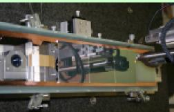
Assembly: Module = 10 GLAST sensors 90 cm strip long
