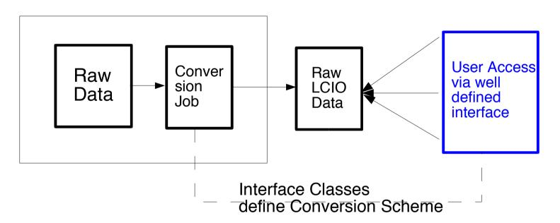
Interface is to be completely decoupled from online software
