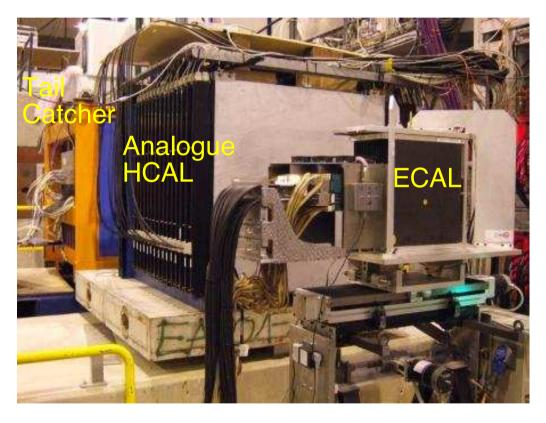
O(15000) calorimeter cells readout by Calice DAQ
