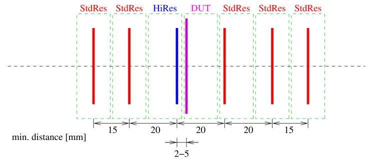
In addition to standard sensor planes with 2  $\mu m$  resolution we can consider adding one high resolution plane ( $\sigma_{HR} \sim 1 \mu m$ ) in front of DUT
