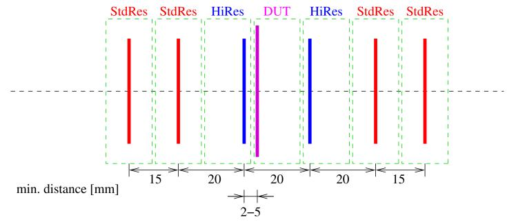
In addition to standard sensor planes with 2  $\mu m$  resolution we can consider adding one or two high resolution planes ( $\sigma_{HR} \sim 1 \mu m$ ) in front of and behind DUT
