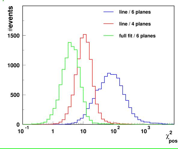
Fit taking into account multiple scattering results in a qualitative improvement in the description of the fitted data.
