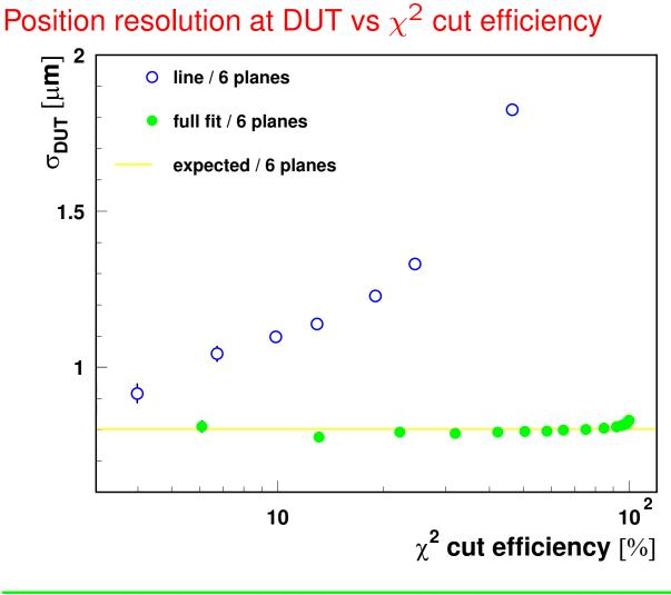
Full fit allows for precise position determination for >90% of events
