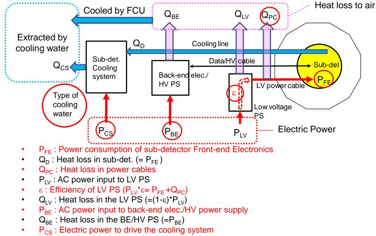
• Q<sub>CS</sub> : Heat to be extracted from cooling system (= Q<sub>D</sub> + P<sub>CS</sub>)
