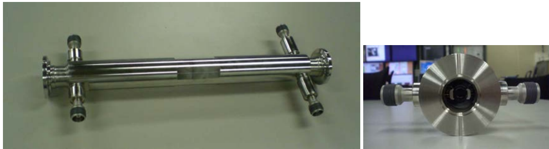
Figure 46: Side view of the stripline kicker
