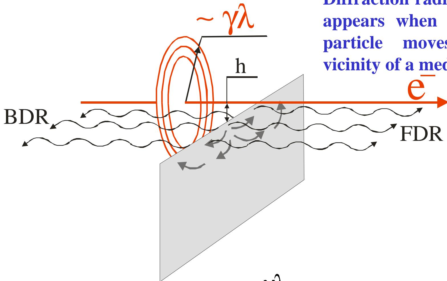
Impact parameter,  $h$ , – the shortest distance between the target and the particle trajectory
