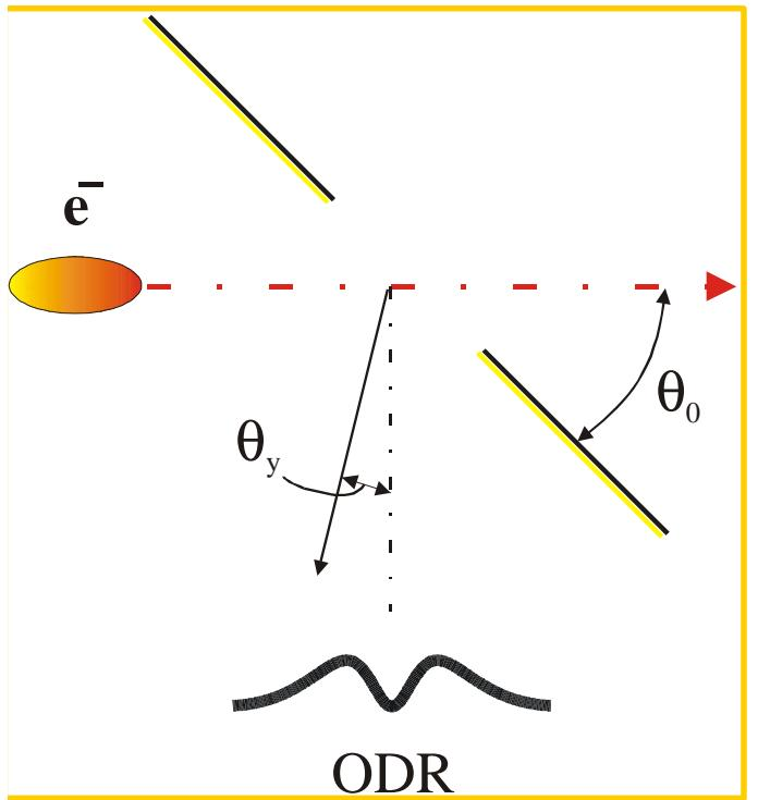
$$\frac{d^2W_y^{\text{slit}}}{d\omega d\Omega} = \frac{\alpha |R_y|^2}{4\pi^2} \exp\left(-\frac{2\pi a_{\text{in}} \sin \theta_0}{\lambda} \sqrt{\gamma^{-2} + \theta_x^2}\right) \times \\ \left\{ \exp\left[\frac{8\pi^2 \sigma_y^2}{\lambda^2} (\gamma^{-2} + \theta_x^2)\right] - \cos\left[\frac{2\pi a \sin \theta_0}{\lambda} \theta_y + 2\psi\right] \right\}$$
