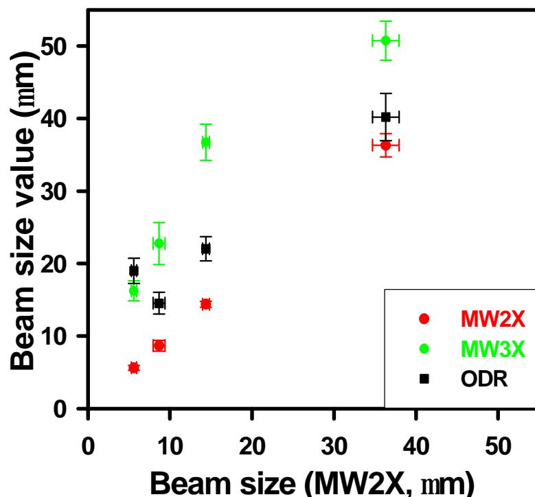
Correlation between the the ODR and the beam size measured with 10mm tungsten wire installed in the target chamber at the same position as the target. The black line represents a 45 degree line.
