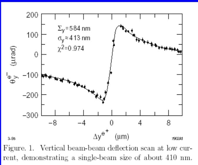
Figure. 1. Vertical beam-beam deflection scan at low current, demonstrating a single-beam size of about 410 nm.
