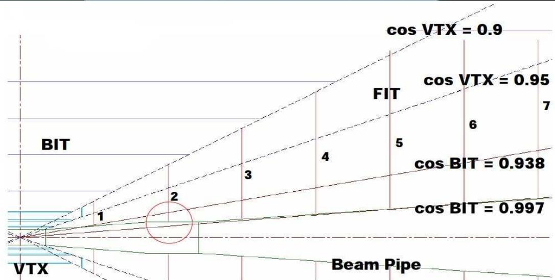
With this tracking system the required momentum resolution of  $\Delta \frac{1}{p} = 5 \cdot 10^{-5} / \text{GeV}$  is reached
