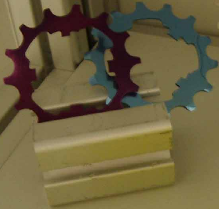
Chemical deburring of titanium crown wheel
